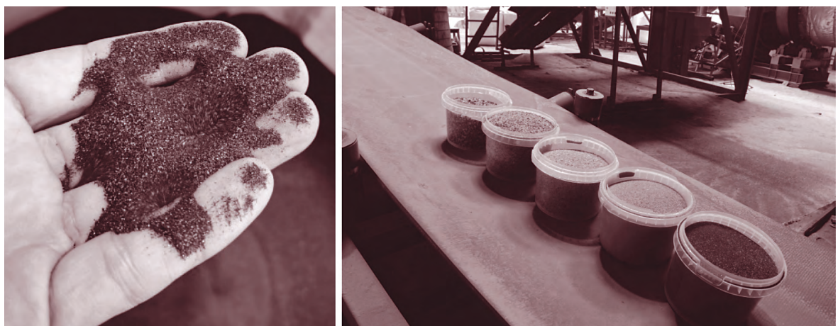
Ilmenite concentrate (raw material for the manufacture of titanium), obtained in the workshop in work settlement Latnaya
